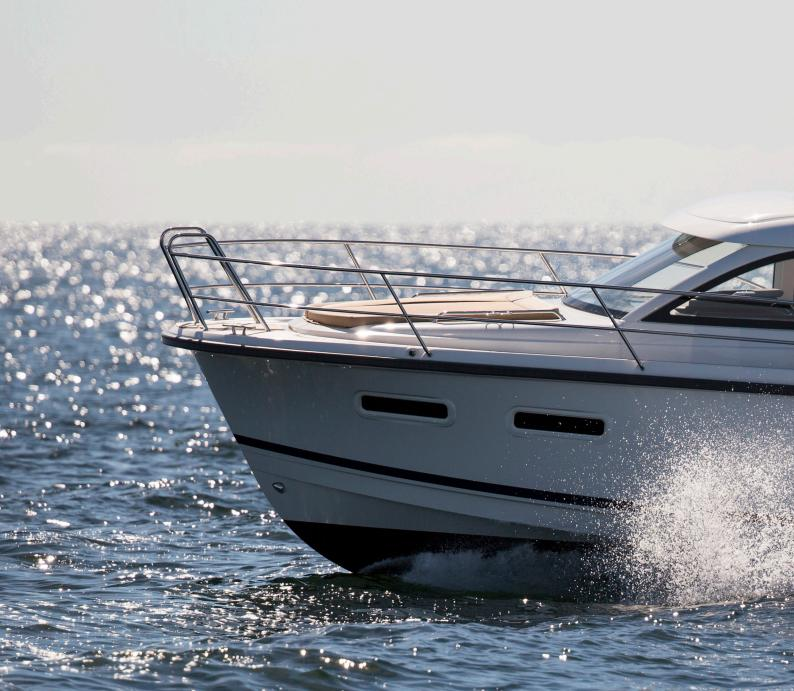
The biggest news is the boat's hull, which has been developed and optimised for speeds from 0 to 22 knots. It is made for smaller engines (Volvo Penta D3), Torqueedo fully Electrical and built to run equally comfortably irrespective of speed. The hydro-dynamic shape of the hull means that the boat has no planing threshold at all.
